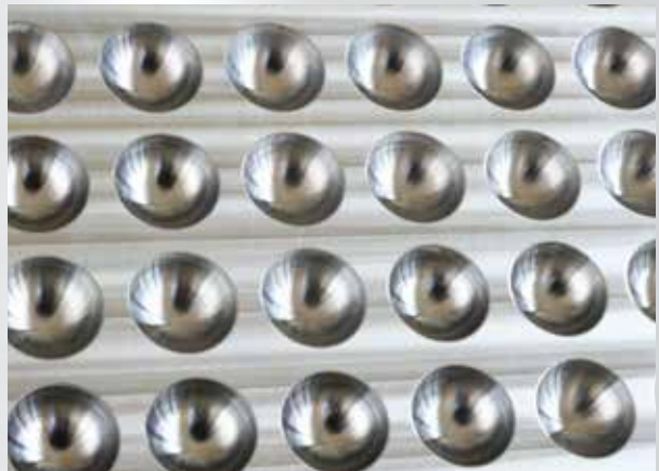
Precision-milled spherical balls ( \varnothing = 5 mm)
